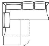
Corner récamière: The seat swivels through 90 degrees beneath the backrest.
